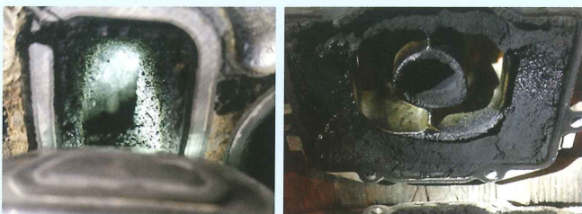
Typical carbon build-ups on air intake system of turbo diesel without Catch-Can protection
